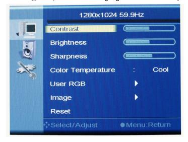
b. Press " $_{\triangle}$ " or " $_{\nabla}$ " to increase or decrease the contrast of the display. Then press "1" to confirm the adjustment and back to OSD main menu.
